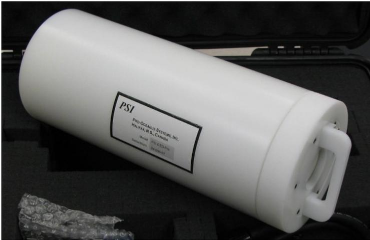
Gas Tension Device (GTD) with Delrin case (approximate length 30cm)
