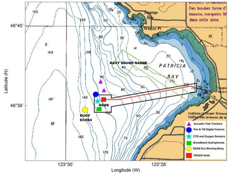
Several instruments have been ordered for use on the VENUS Observatory in Saanich Inlet. The majority of these sensors will reside on a bottom-mounted platform located within a few hundred meters of the node. This platform will house a SIIM (Scientific Instrument Interface Module), into which the following devices will be plugged:
