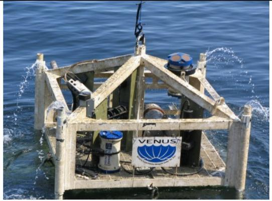
**Figure 4:** The VIP being recovered after 6 months at 95 m in Saanich Inlet.
