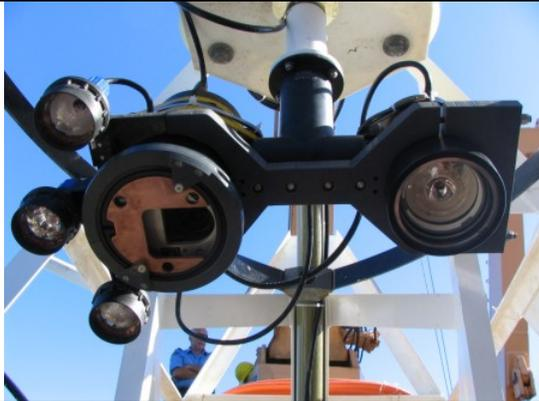
**Figure 3:** The camera system just before re-deployment. A new TTL flash was installed.
