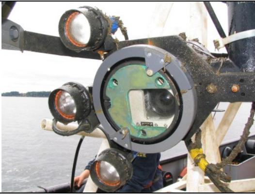
**Figure 1:** The camera window after 6 months at 100 m in Saanich Inlet.
