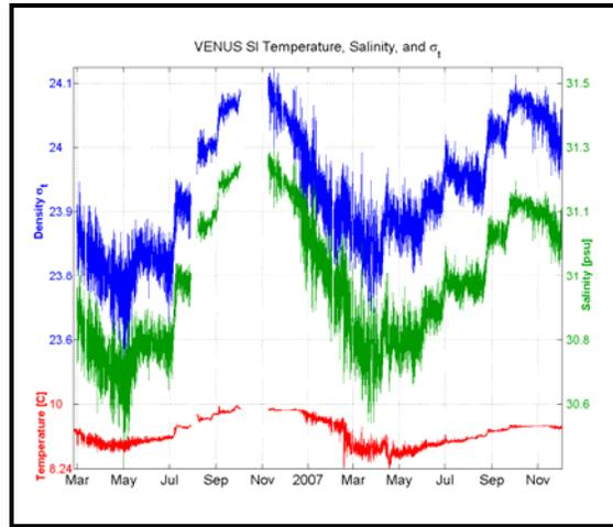
**Figure 2.** Time series of temperature [red], Salinity [green], and  $\sigma_t$  [blue, density(T,S,0)-1000] from the Saanich Inlet SBE CTD at 96 m depth on the VIP for Feb. 2006 – Dec. 2007 (UTC). Temperature has been scaled to show its (minor) contribution to density relative to salinity.
