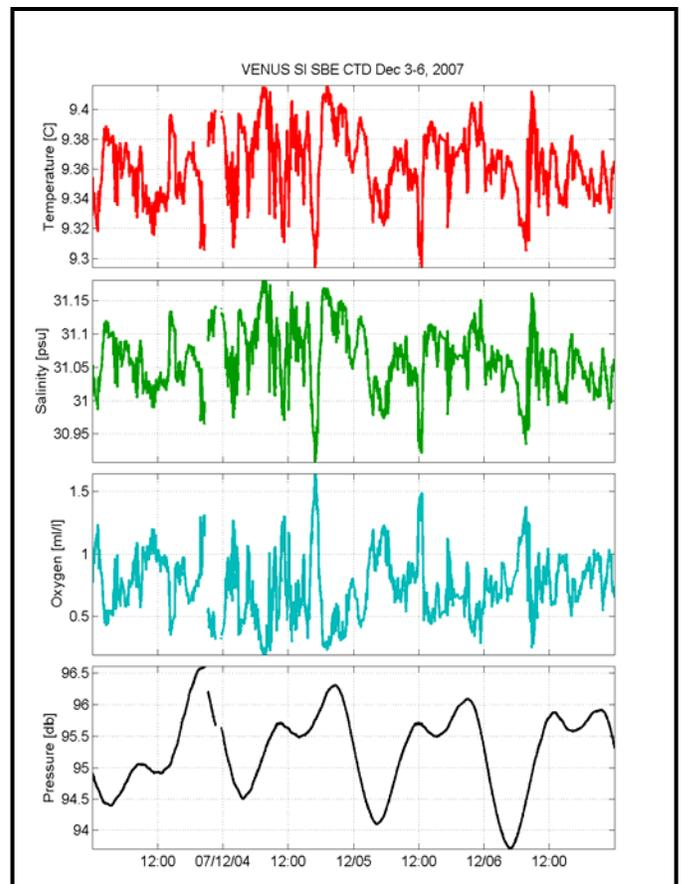
**Figure 1.** Time series of temperature (red), salinity (green), oxygen concentration (cyan), and pressure (black) from the Saanich Inlet SBE CTD at 96m depth on the VIP for December 3-7, 2007 (UTC). Short gaps in the data late on Dec. 3 were a result of a winter storm causing a power outage at IOS.
