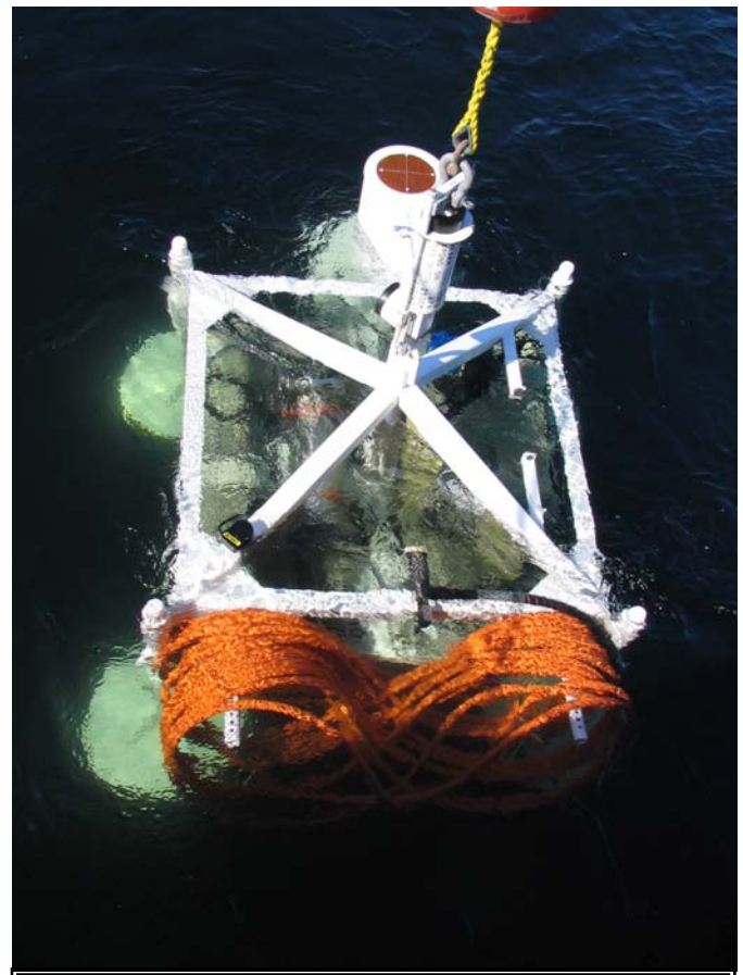
The instrument platform being redeployed in Saanich Inlet. The real-time sediment trap is on the top, just behind the lifting line. For the full story on the Saanich Inlet Maintenance Cruise, please see Page 2.
