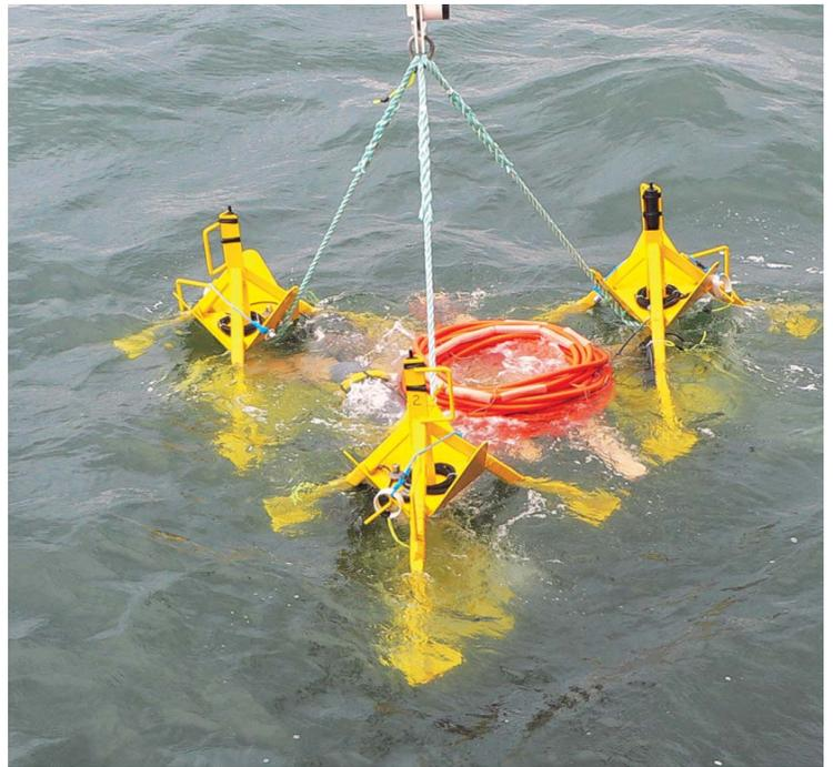
Strait of Georgia Hydrophone Array being deployed to 300m
