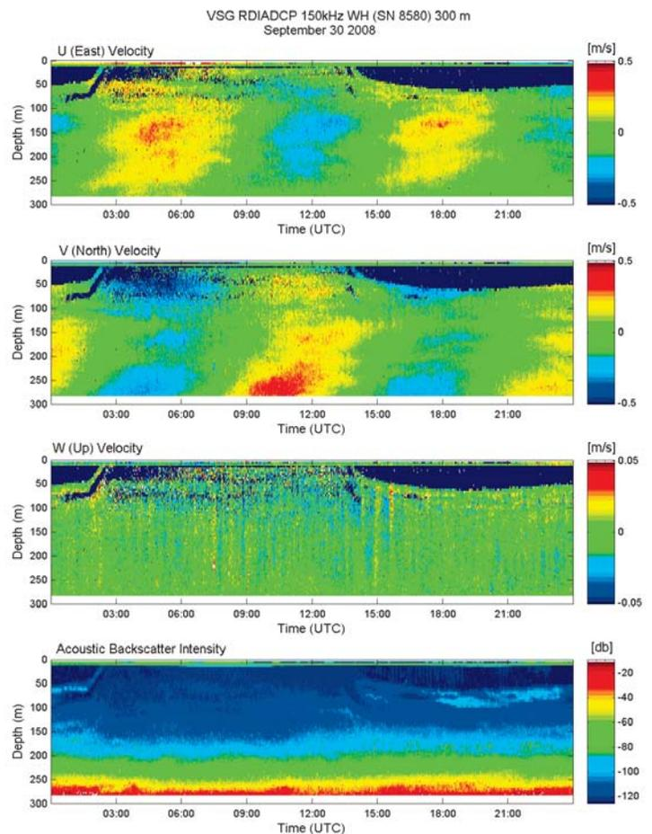
Figure 3 RDI ADCP 150kHz WH (SN 8580) data from September 30 2008. U, V, W velocities and Acoustic Backscatter Intensity
