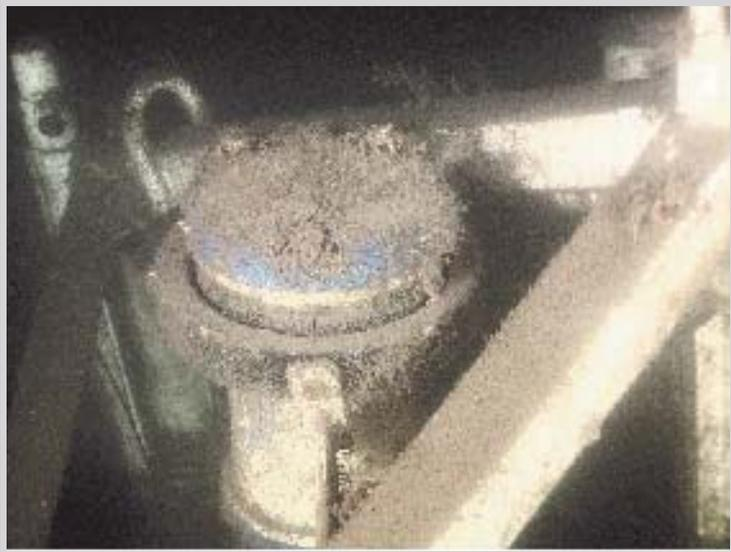
Figure 1. ADCP on DDL after 6 months
