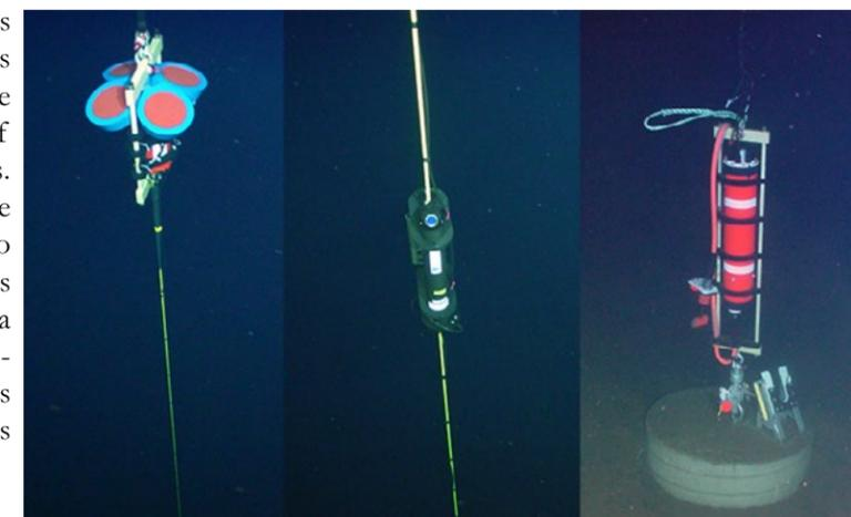
*The RCM is composed of three different types of instruments affixed at varying depths along a cable extending from the seafloor upward 267m. Above (from left to right): 75 kHz Acoustic Doppler Current Profiler (ADCP), collocated CTDs and ACMs, mooring base and 650kg anchor weight on seafloor.*
