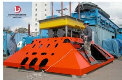
*Above, ROV serviceable science node being lowered into trawl resistant frame*
